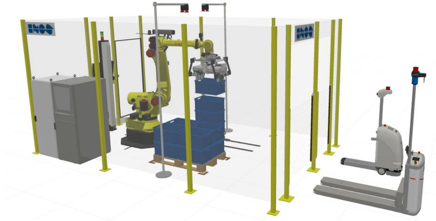
Material handling between AGV-Systems (Dolly to pallet)
