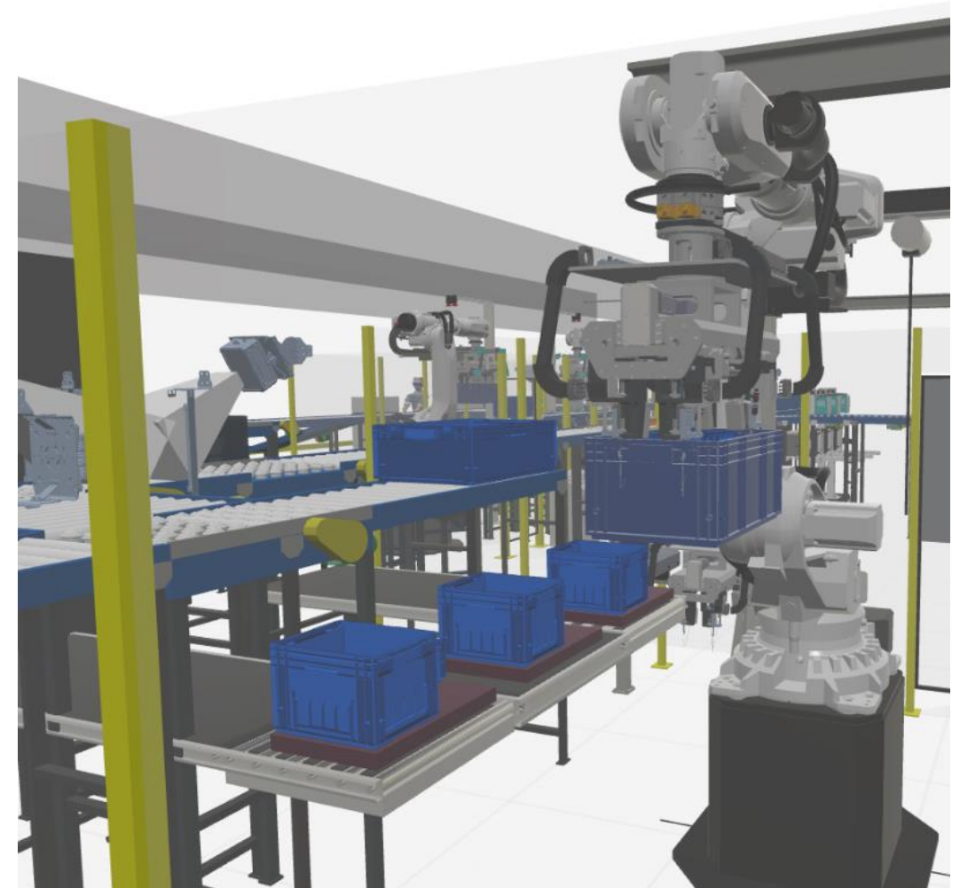
De-Pallettizing of different boxes with change of grippers / identification of empty boxes / De-Palletizing from Trays
