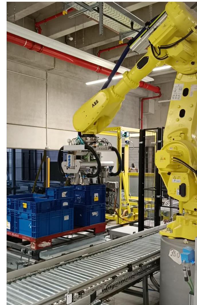
inos KLT Standard Handling solution with Flex-Gripper at OEM
