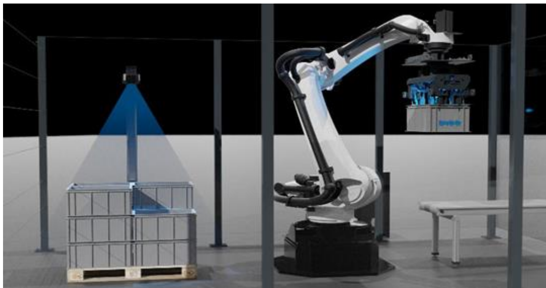
inos KLT Standard Handling solution with Flex-Gripper and Vision system
